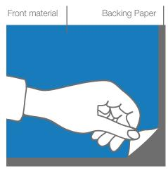
Backing Paper is slightly larger than Front material. Avoids adhesive bleeding, no adhesive residues in the printer.
