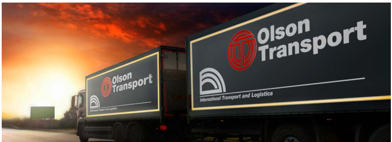
Avery Dennison V-4000 E applied on truck trailer in accordance with regulation ECE104.
