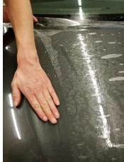
When using Avery Dennison Pure Defense PU and PVC, re-positioning of the film is only possible in the stage of initial positioning and low or no squeegee pressure. If done in a later stage small marks or lines might remain visible in the film surfaces.
