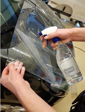
Remove the liner and spray the exposed adhesive side with the soap solution. Then position the material on the selected application area. If necessary, slide the film until you have reached the
