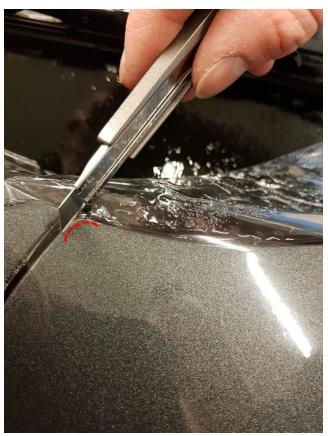
To facilitate cutting, make sure to use a new and very sharp knives for cutting: dull knives will result in blurred cutting edges. When applying Avery Dennison Pure Defense PU and PVC, it is recommended to use stainless steel blades with your knife. The use of stainless steel blade will delay rusting and deterioration of the blades, due to contact with water.
