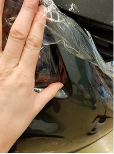
Avery Dennison Pure Defense PU presents a good degree of conformability, thus conventional convex and compound shapes on car fronts are mostly suitable to be covered with this film. Nevertheless, in deep corrugated shapes, it may be necessary to make an incision in order to avoid any form of air/water entrapment in the deep recesses. This incision does not jeopardize the functionality or durability of Avery Dennison Pure Defense PU.
